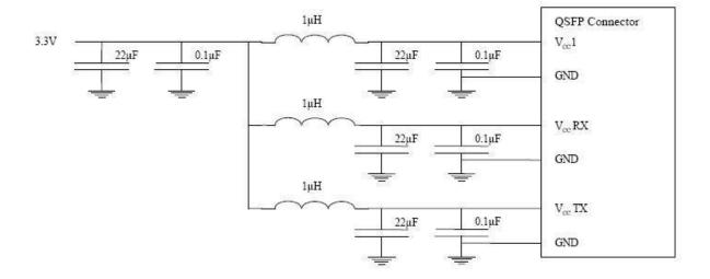
**Host Board Power Supply Filtering**
